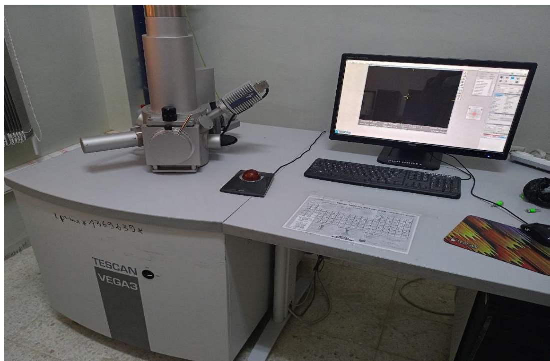
Figure II.2: Bruker Nano GmbH scanning electron microscope (SEM) equipped with an energy-dispersive X-ray spectrometer (EDS). (Biskra university)
