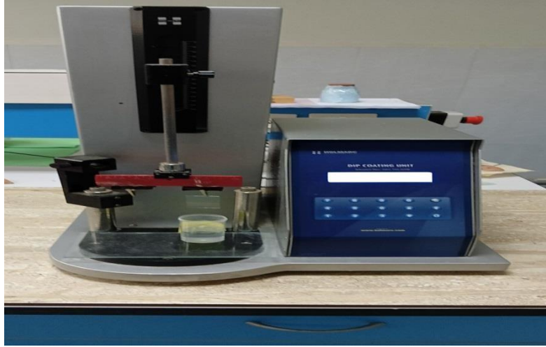
Figure II.2. Holmarc's sol gel dip-coating method.
