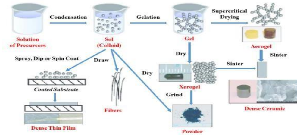
Figure II.1. Main steps of the growth of thin films by sol-gel method [6].
