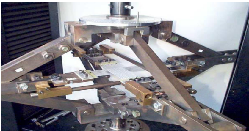
Figure (2.14) Dispositif de traction biaxial [10].
