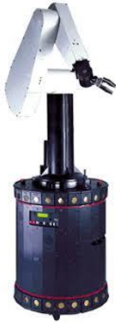
Figure I.10. Le robot omnidirectionnel Nomadic XR4000.
