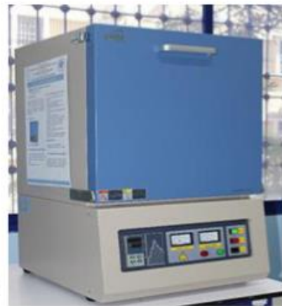
Figure II.22: Cycle de traitement de calcination. Figure II.23: Four de calcination.
