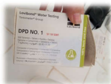
Figure 35 : test de chlore.
