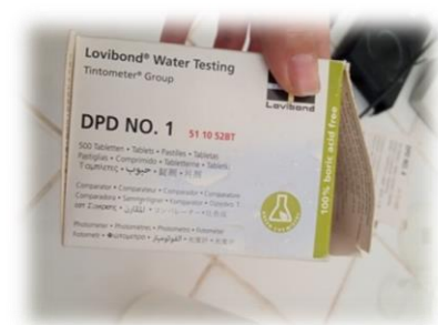
Figure 35 : test de chlore.
