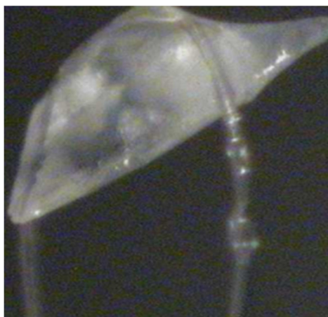
Figure 7: Monocristal transparent du composé (BCFF).
