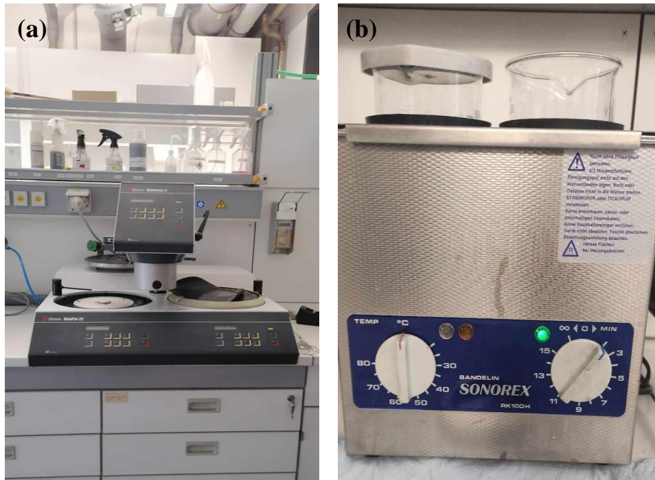
Figure II.10: (a) Polishing machine; (b) Ultrasonic bath.
