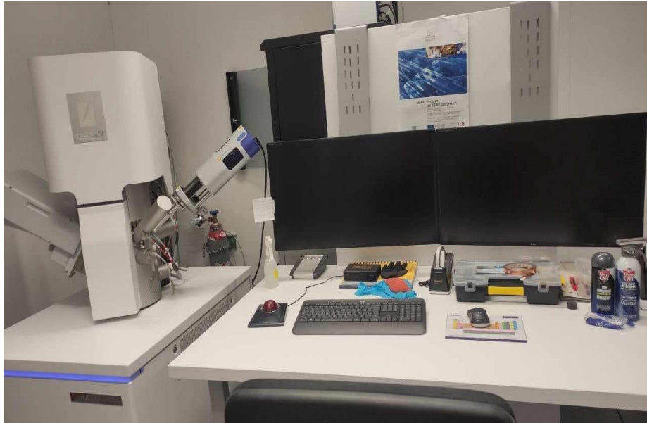
Figure II.9: Scanning electron microscopy (SEM) machine type TESCAN MIRA, Germany.
