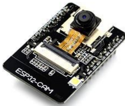
Figure II.3 : Carte ESP 32-CAM
