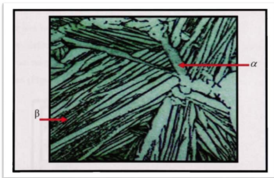
Figure 21: Exemple microstructure lamellaire [56]
