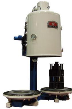
Figure II.5. Four de nitruration plasma [8].
