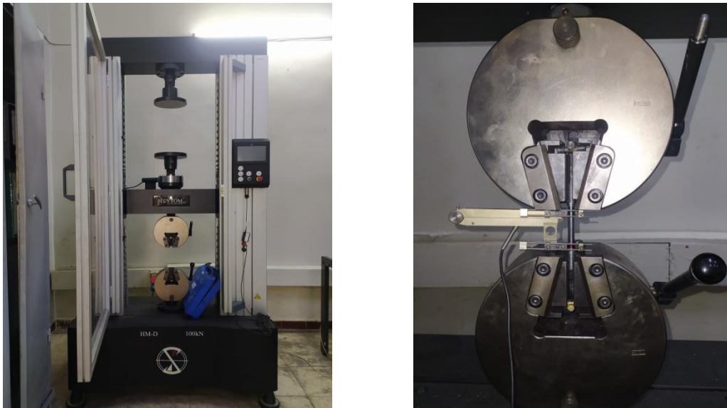
Figure III.16. Machine de l'essai de traction.
