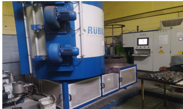
Figure II.3. Four de nitruration gazeuse [11].
