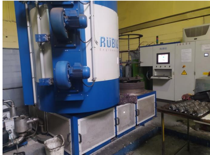
Figure III.5. Four de nitruration gazeuse.
