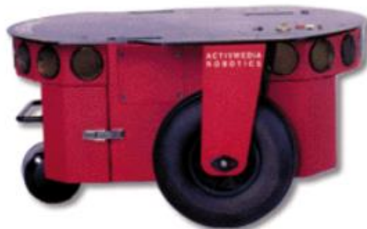
Figure II.6. Robot mobile Pioneer P3-DX , ActiveMedia Robotics, 2004 [20].
