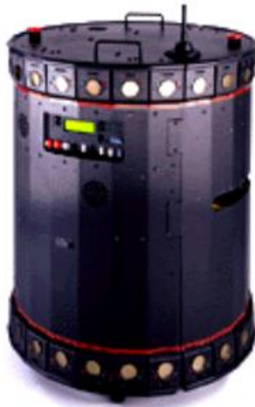
Figure II.14. Robot mobile omnidirectionnel Nomadic XR4000.
