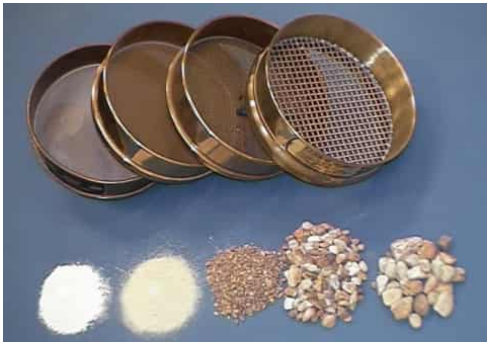
Figure 2.1: Soil types with particle sizes. Shown (right to left): medium gravel (9.5-mm), fine gravel (2.0-mm), medium-coarse sand (0.425 mm), silt, and clay (0.075 mm) (Samtani et al. [68]).
