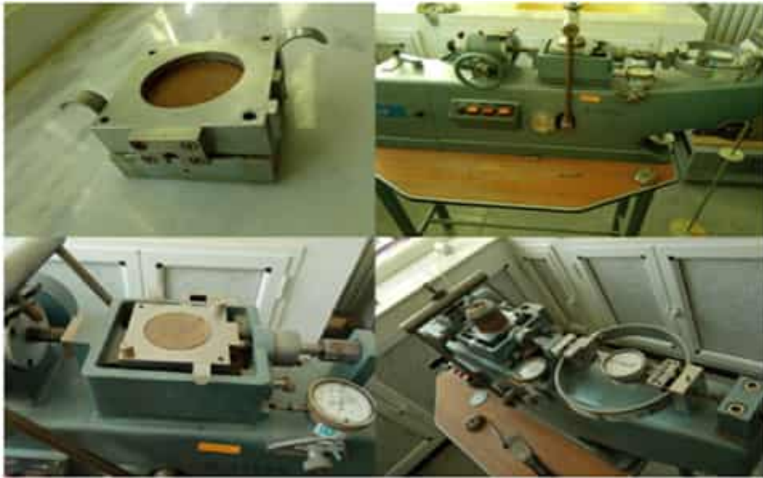
Figure 3.3: Direct shear test apparatus used for determining shear strength parameters of the clayey sand.
