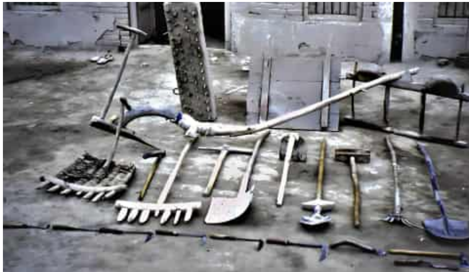
Figure 1.2: Traditional agricultural and excavation hand tools shovels, spades, picks, and mattocks commonly used for small scale manual excavation and soil preparation (Thomas [38]).
