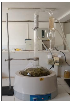
Figure 18 : Montage hydrodistillation clevenger
