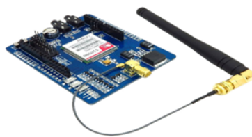
FIGURE III.11 – Shield GSM SIM900.
