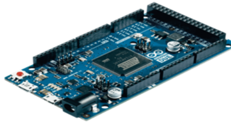
FIGURE III.6 – Carte Arduino DUE.
