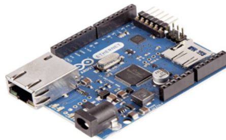
FIGURE III.2 – Carte Arduino Ethernet.
