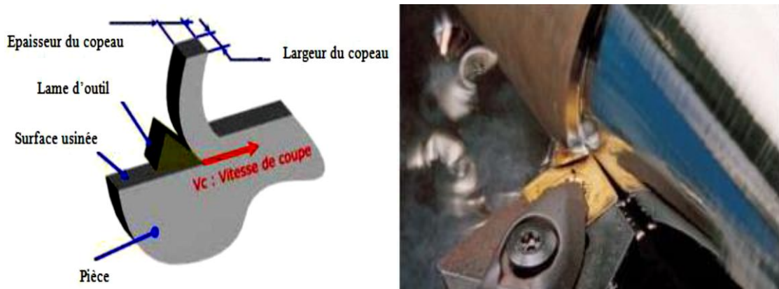
Figure I- 2. Principe de tournage [6].
