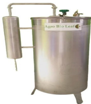
Figure 3. Extraction equipment Hydro steam distillation apparatus
