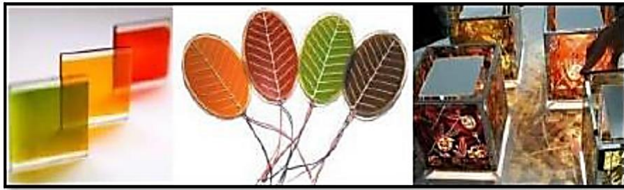
Figure I.16: Cellules solaires à colorant [22]
