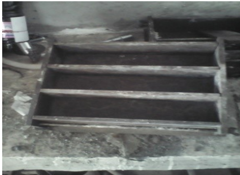
FIGURE III.7 — Epreuves prismatiques (7x7x28).
