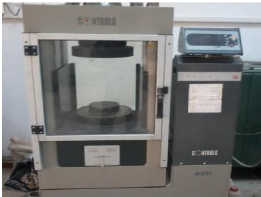
FIGURE III.9 — Presse hydraulique de compression.
