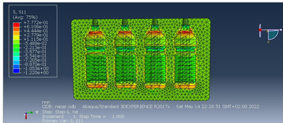
Figure III-8 : La concentration de la contrainte axiale \sigma_{XX}
