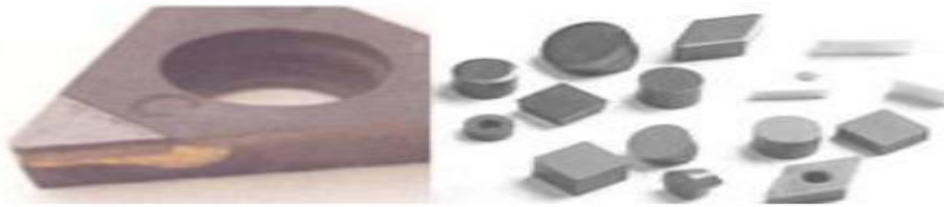
Figure I-28 : Les diamants poly cristallins. [28]
