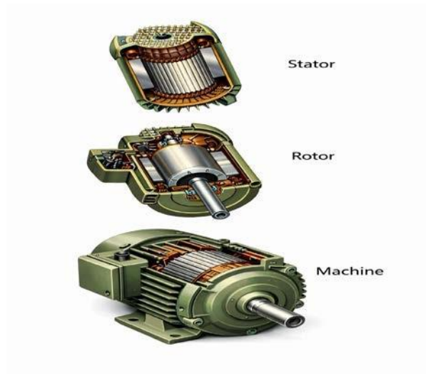
Fig.I.1: Construction de la machine asynchrone
