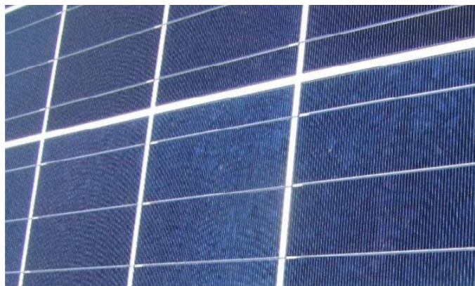
Figure 12:Module de silicium poly cristalline
