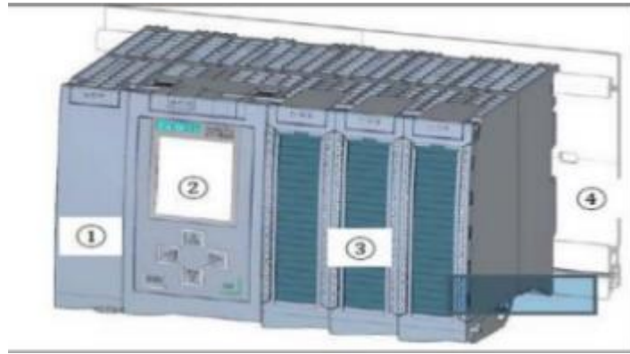
Figure II.11: Structure d'un automate S7-1500
