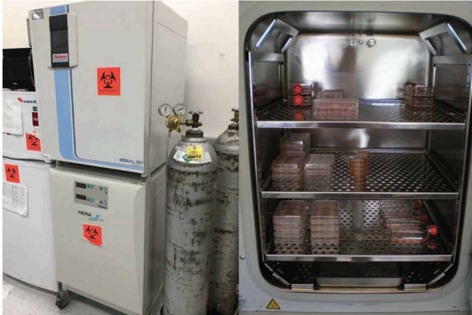
Figure 25. Left: double-stacked CO 2 incubator with a CO 2 gas tank attached to it; right: multiple cell culture flasks within a CO 2 incubator (Yoon, 2022).
