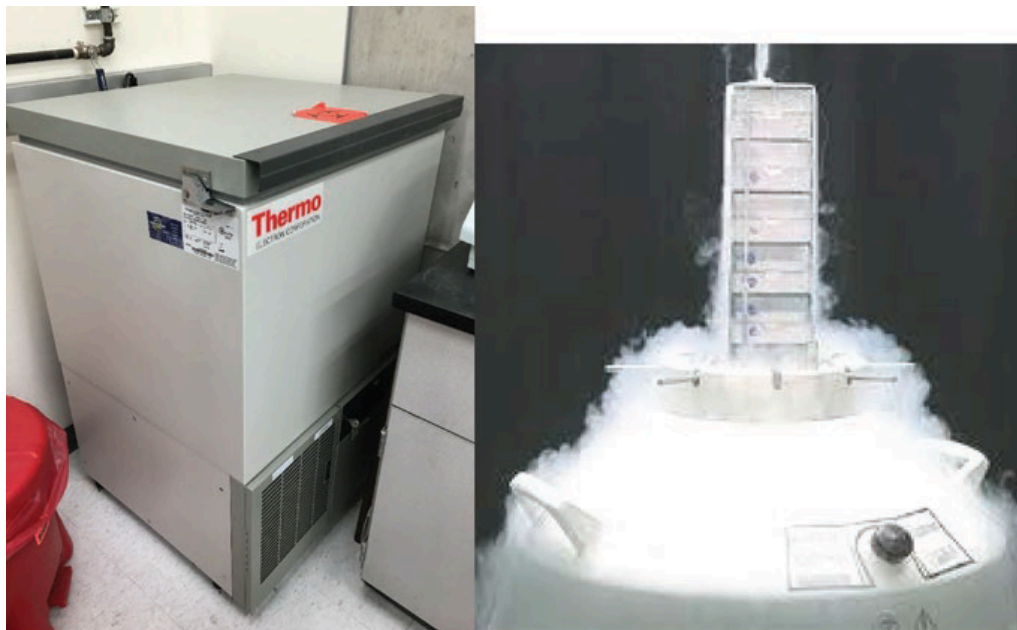
Figure 28. -40^{\circ}\text{C} deep freezer (left) and liquid nitrogen tank (right) for storing mammalian cells (Yoon, 2022).
