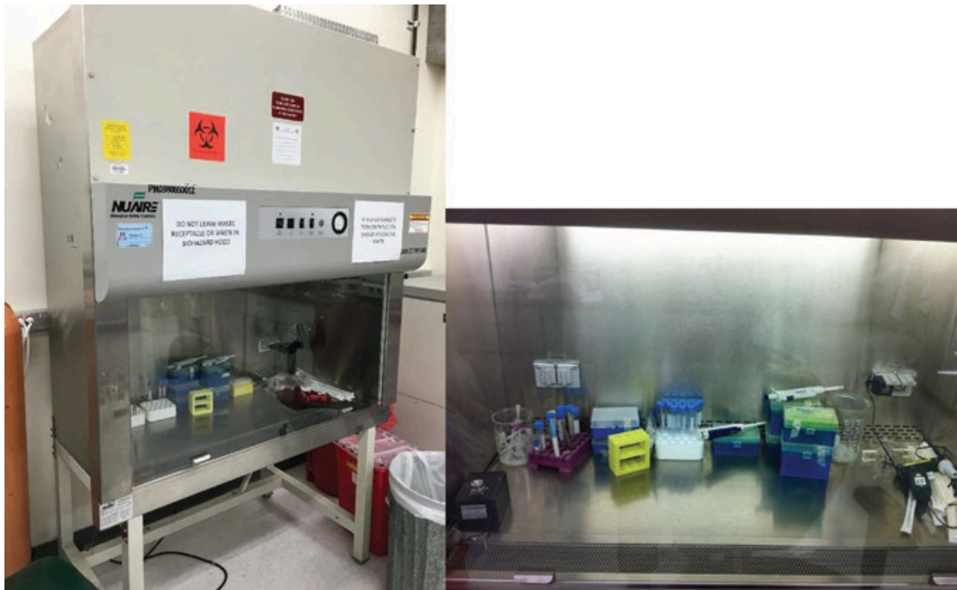
Figure 24. A class II biosafety cabinet: (left) overall view and (right) inside view (Yoon, 2022).
