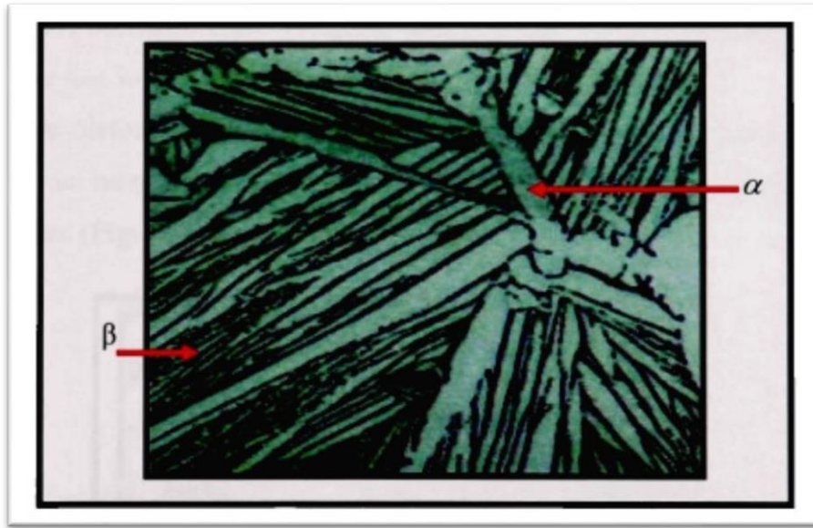
Figure 1.21: Exemple microstructure lamellaire [56]
