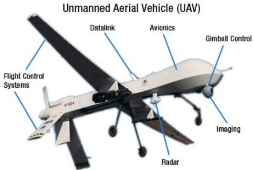
Figure I.18. Various devices and sensors mounted on a UAV.
