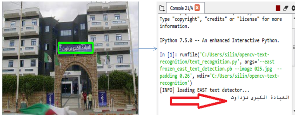
Figure 5.8: Test Images Contains a Arabic Words and The Console Results.
