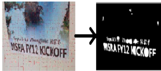
Figure 3.1: Example of MSER Text Detection.
