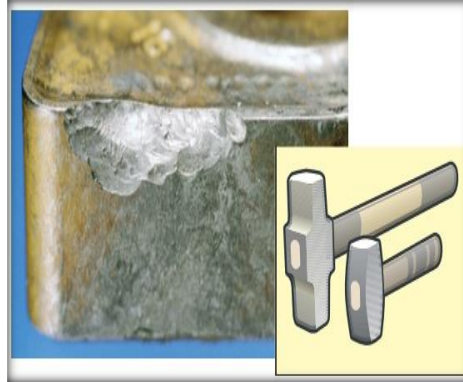
Figure II.31 : Usure mécanique (Ecaillage).
