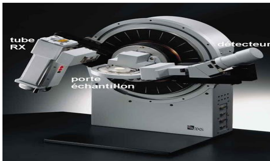
Figure II.6 : Diffraction des Rayons X – DRX. [9]
