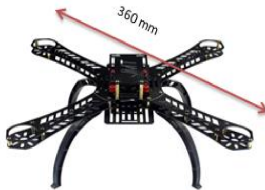
Figure III.2: Frame (carbon fibre)
