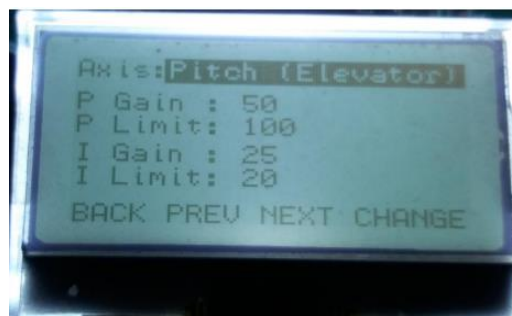
Figure III.18: Inside the PI Editor Menu and adjusting the Pitch Axis PI values for Stable Flight Channel : 2
