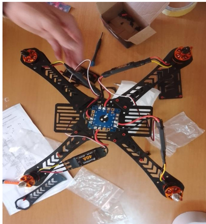
Figure III.31: The installation of engines and ESC
