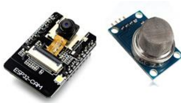
Figure III.34: Smoke Sensor m-Q135 with camera esp 32
