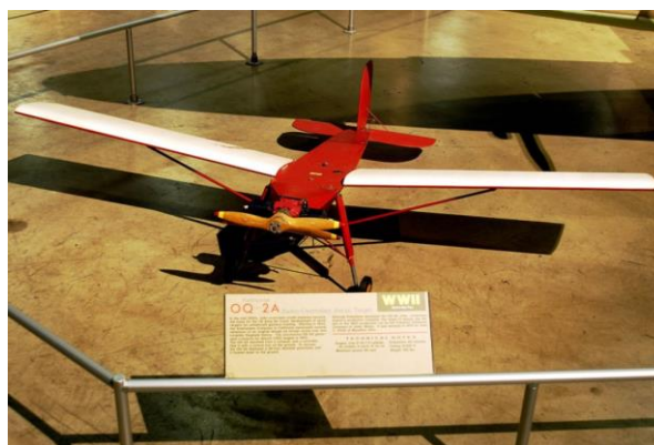
Figure I.4: The OQ-2 Radio plane was the first mass- Produced UAV or drone in the United States ,
