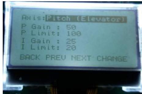
Figure III.17: Inside the PI Editor Menu and adjusting the Pitch Axis PI values for Stable Flight Channel : 1
