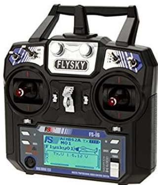
Figure III.27: remot control flysky fs-i6
