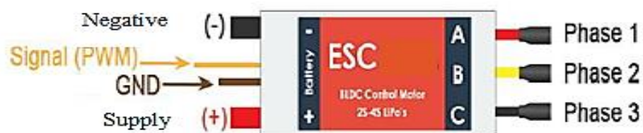
Figure III.11 : Electrical Speed Controllers (ESC) scheme
