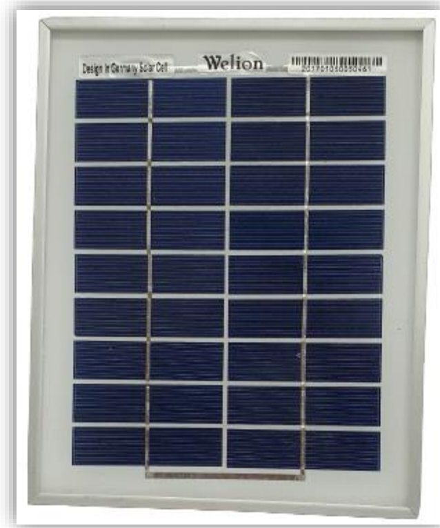
Figure III.4 : Panneau solaire 5W - 9V (Welion)
