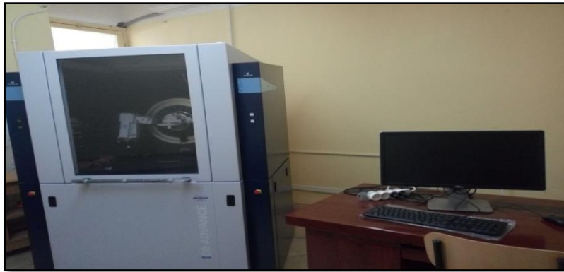
Figure III.13: Photo de l'appareil DRX (Bruker D8).
