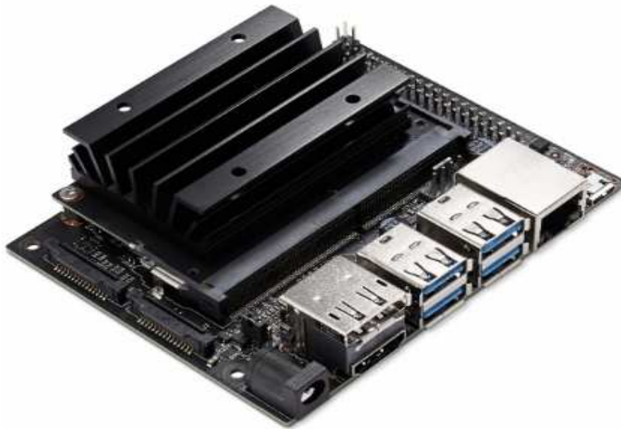
Figure IV. 3. NVIDIA Jetson NanoB01.
