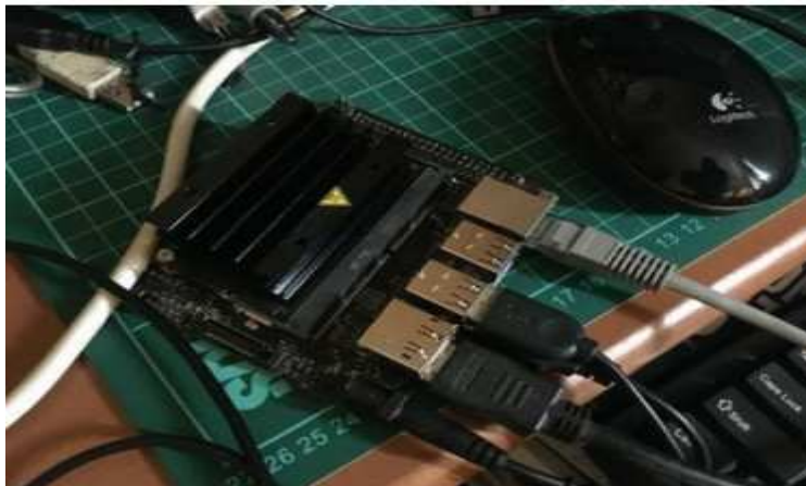
Figure IV. 5. Connecting a UTP LAN cable to a NVIDIA Jetson Nano.
