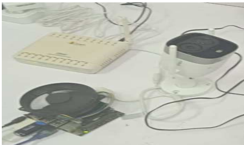
Figure IV. 21. Connecting the Nvidia Jetson Nano and the IP Camera.
