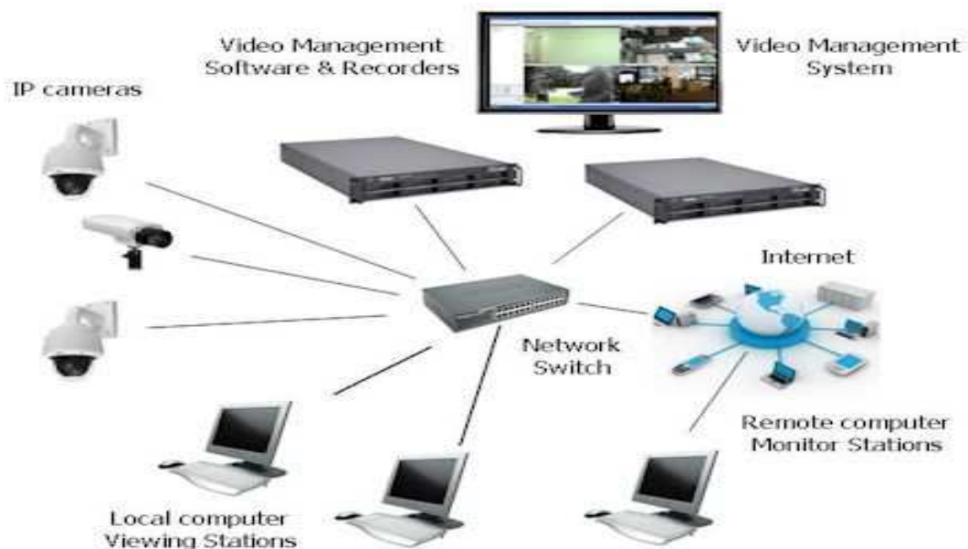
Figure I. 3. IP CCTV cameras diagram.
