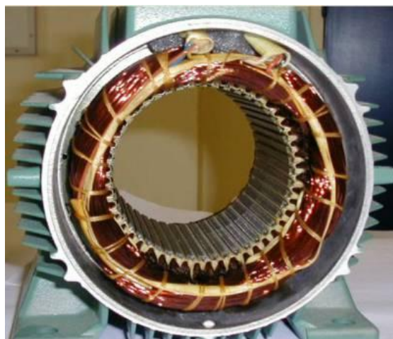
Figure(I.2): Stator de la machine asynchrone
