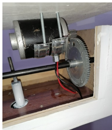
Figure 48: Gear train mounted on the shaft mating with generator
