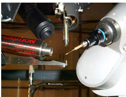
Figure II.15 : Diffraction RX sur monocristal
