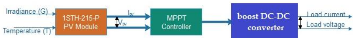
Figure IV.1. MPPT system using 1Soltech 1STH-215-P PV Panel
