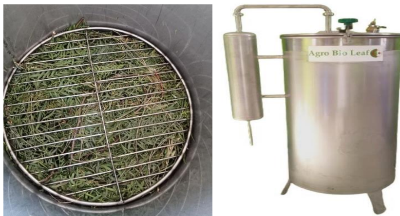
Figure 14. Extraction equipment, Hydro steam distillation apparatus from the inside and the outside (Original photo, 2024)
