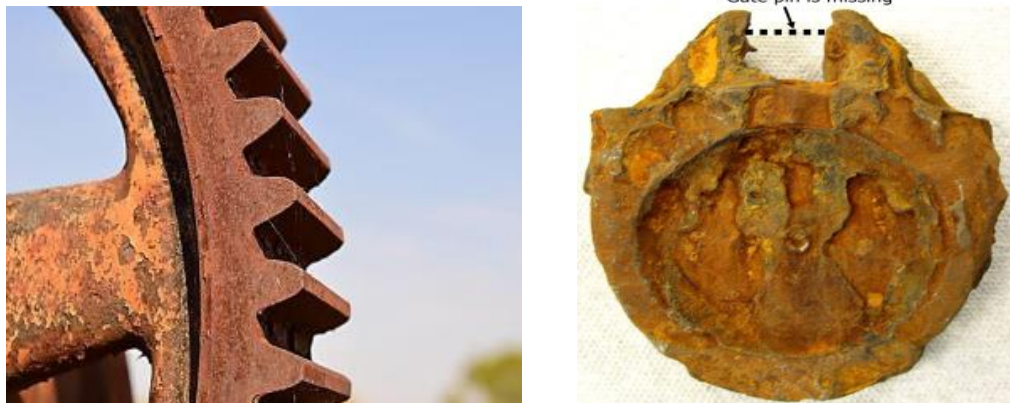
Figure (I.3) : Corrosion uniforme.
