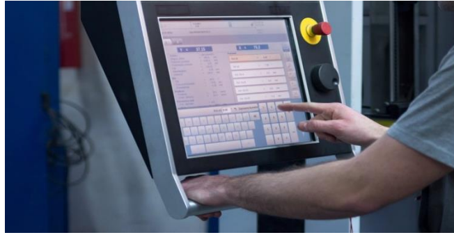
Figure II.5: exemple de HMI
