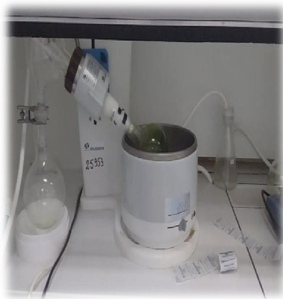
Figure 37: Evaporation le filtrat.
