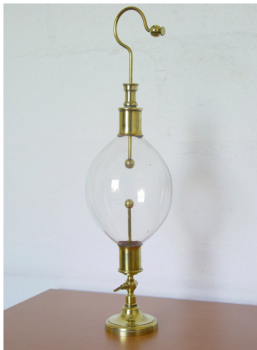
Figure II.1: Appareil de Faraday
