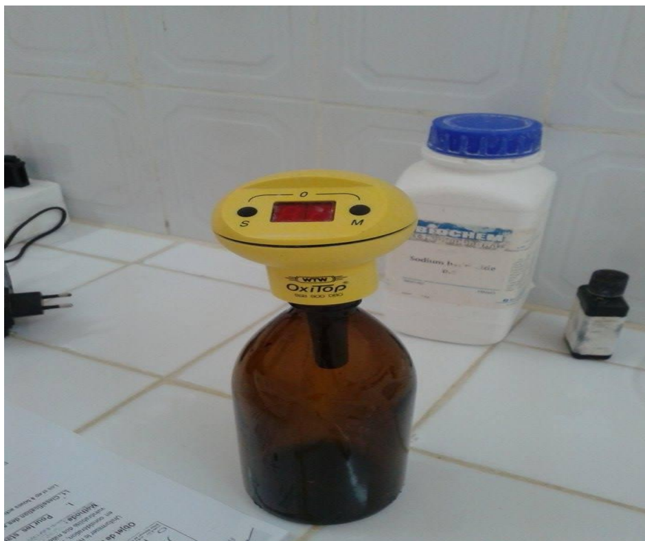
Figure III.10 : Oxytop / 6 postes wtw
