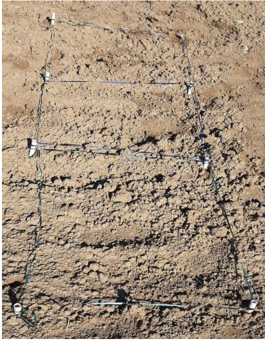
Fig. 06: Three areas of one 1 M 2 were irrigated for 45 a days (ones every 7days)
