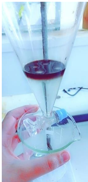
Figure II.7: Extraction de la caféine
