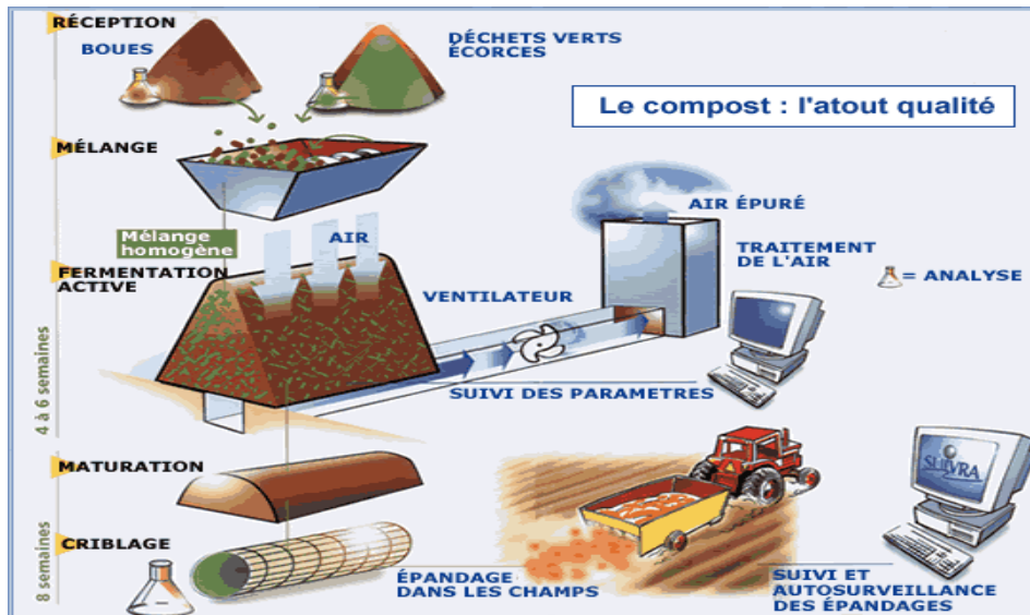
Figure 26 : Processus de compostage source internet
