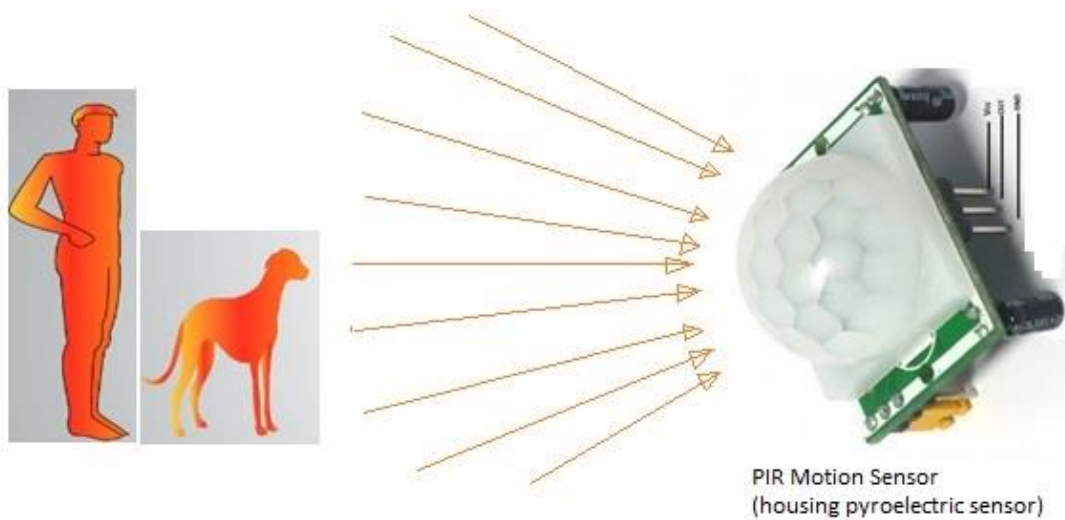
Pic30 .....how pir sensor works
