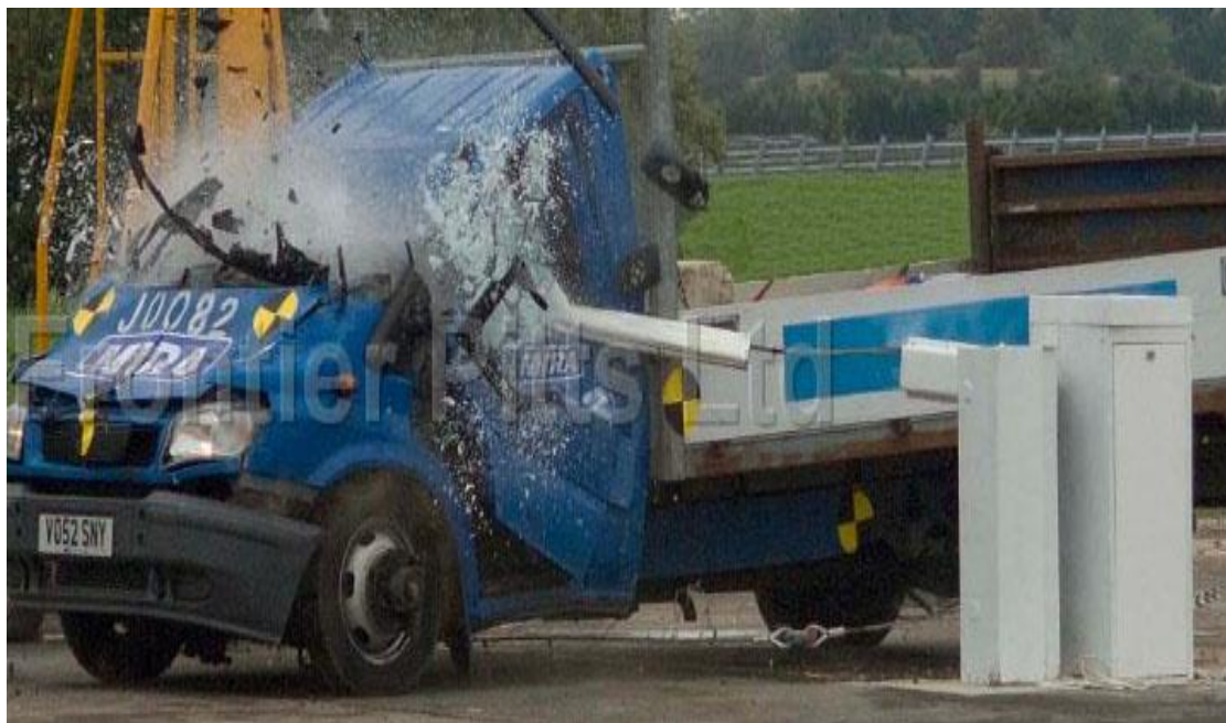
Pic 13 .....truck hit a TERRA COMPACT barrier
