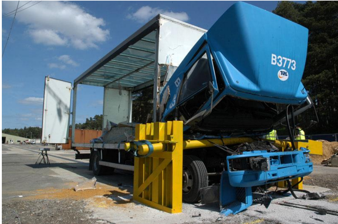
Pic 7 .....a truck hit a TERRA-Manual barrier
