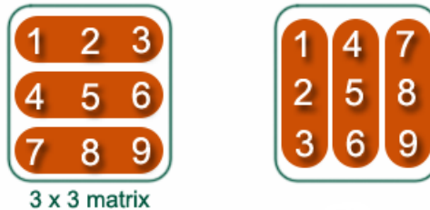
Figure 5.2: An example of a 2-D array.
