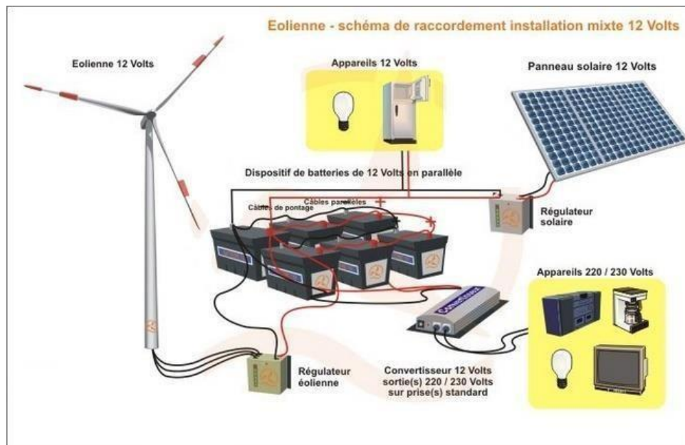
Figure I.04 : Installation photovoltaïque hybride [4].
